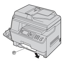
3. Insert the standard input tray into the unit, lifting the front part of the tray. Then push it completely into the unit.
